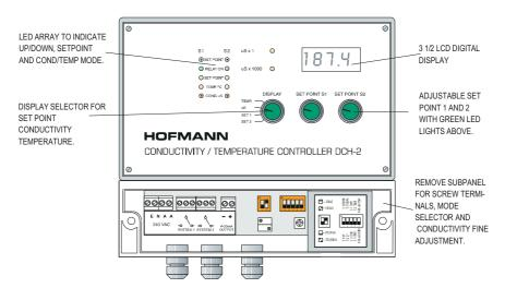
FIG.2 FRONT PANEL LAYOUT
