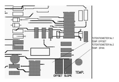
FIG.13 ADJUSTMENTS FOR TEMPERATURE
